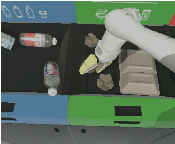
Figure 3. In the simulated vision-based robotic grasping tasks, a robot arm must grasp various objects placed in bins in front of it. Full implementation details are described in Appendix A.1.2.
